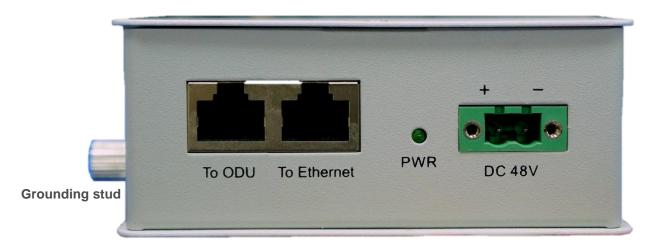
**Power Over Ethernet Injector Figure**
