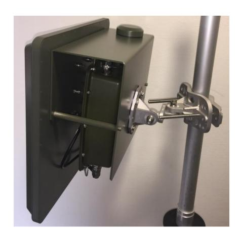
NATO Radio link 4.4/4.99 GHZ 2x2 MIMO 2x100 watts EIRP.
